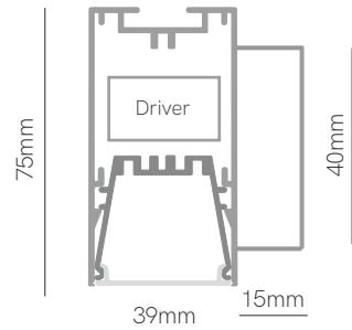
\*Finished luminaire. Includes power supply, base wall and end caps.
